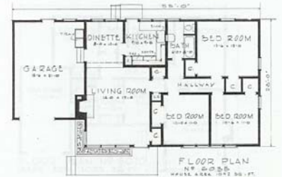
PLAN NO. 6035—Low sweeping roof lines and corner windows are the feature of this modern three-bedroom home all on one floor. No basement is needed where space for the laundry and heating plant is provided in attached garage.
