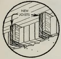
Brick or concrete blocks are packed into the spaces between the 10" and 12" joists; they are supported by the plywood panels.
