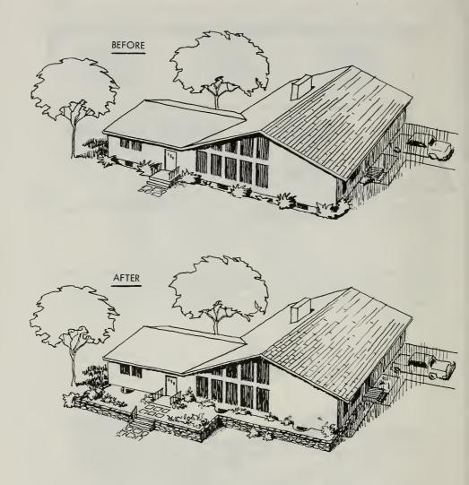
Where basements are not completely belowgrade, here are some additional ideas which can be used to increase the shielding of exposed basement walls. A brick, masonry, or stone planter box along one or more sides of the house will improve protection substantially, and will provide an attractive setting for shrubs and flowers as well. If the partially exposed wall is at the rear or side of the house, an elevated garden could be built with masonry retaining walls.
