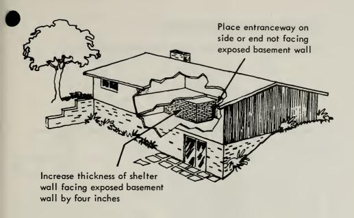
If your basement ceiling is near ground level on three sides and exposed on one side (as with "walk-in" basements), the concrete block shelter (Plan C) must be modified to achieve the desired effectiveness. The following changes should be made:
