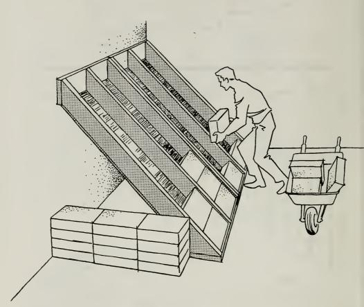
A simple and effective lean-to shelter can be built by constructing the components and storing them in your basement where they can be quickly assembled in an emergency. Components consist of a frame and filler materials, such as brick or blocks.
