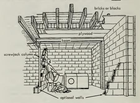
Here is a shelter which can be permanently installed in the basement of your home without affecting the use of the basement in any way.
