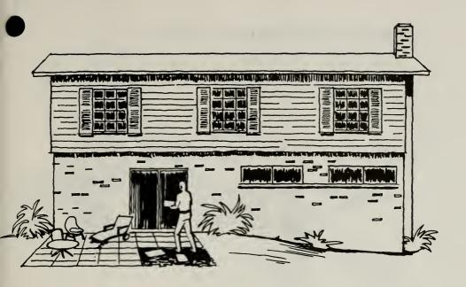
A patio of brick or concrete block supported on a bed of sand will provide a ready source of shielding material which could be quickly removed for use in an emergency. See Plans D, E and F.
