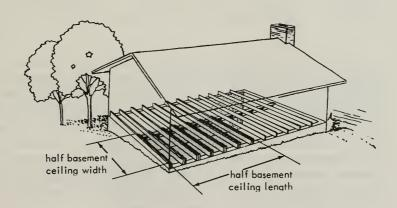
This basement floor plan shows how the additional joists and the filler material might be used in the corner of the basement which furnishes the best fallout protection. To get the most protection out of this improvement, one-quarter of the basement ceiling should be filled with bricks or solid concrete blocks.
