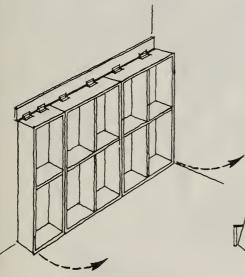
A tilt-up storage unit in a corner of your basement is another approach similar to the snack bar. The top of the storage unit can be hinged to the wall and the unit can be used as a bookcase, pantry shelves, or for miscellaneous storage.
