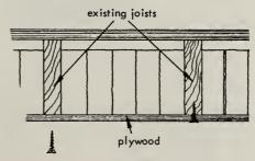
In fastening the plywood sheets to the joists, nailing is not enough. Nails will pull loose. Use two-inch screws in the manner shown here.
