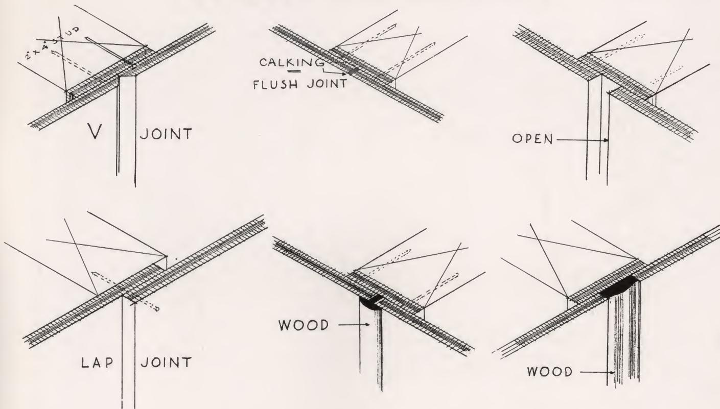
Furring sticks should be cut of  $\frac{1}{4}$ " plywood two inches wide with the grain running the short way of the stick. Nail sticks to studs and girts. For best results, panels should be glued and nailed to the furring. Nails can be used alone if necessary.
