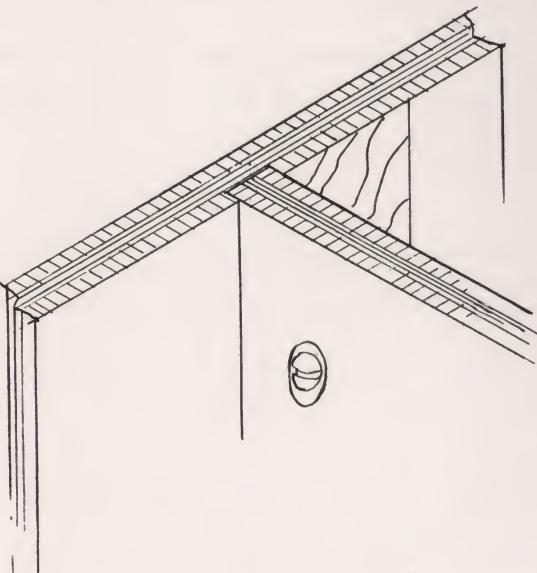
construction which is necessary when plaster or other materials with less strength than plywood are used. It is possible to build closets and storage units in the manner illustrated out of single thickness plywood without studs. An obvious advantage of this system is illustrated in the double faced kitchen cabinet units. The illustration demonstrates how the inaccessible corners in kitchens may be utilized for storage cabinets and shelves in adjoining rooms.
