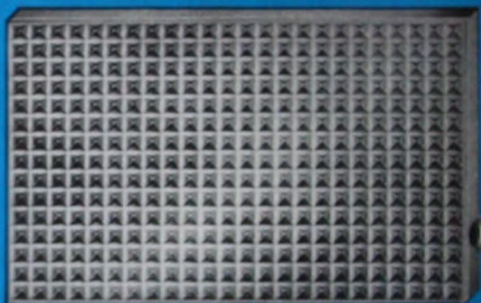
REGLEX GLASS • (Pattern Shown Actual Size.) A popular pattern for the interior glazing of fine buildings. The design is made of pyramidal-shaped indentations—64 to the square inch—which diffuse the light remarkably well and at the same time provide great obscurity. (See table of Sizes, Thicknesses, etc.)
