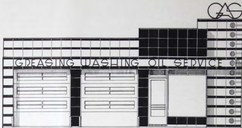
GAS AND SERVICE STATION SHOWING EFFECTIVE APPLICATION OF VITROLITE CEMENTED TO MASONRY WALL • SCALE 1/8"=1'-0"
