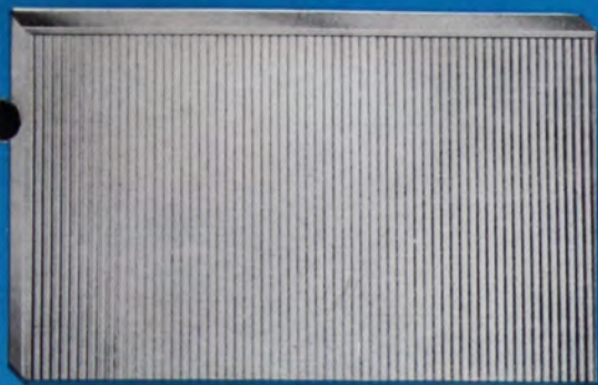
RIBBED GLASS * (Pattern Shown Actual Size.) Used only for industrial glazing. Diffuses light when clean but has a tendency to collect dirt more rapidly than our newer patterns. Available both plain and wired. (See table of Sizes, Thicknesses, etc.)
