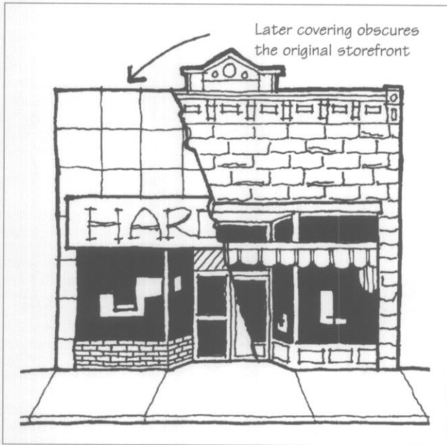
Don't cover or obscure original facade materials.
