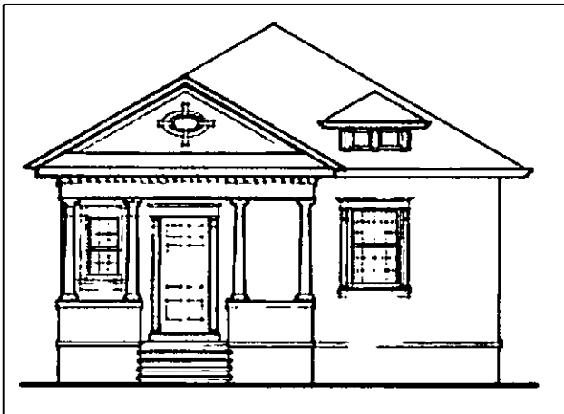
Preferred Approach, when historical documentation is available: Neoclassical style house with a replacement porch designed similar to that seen historically.
