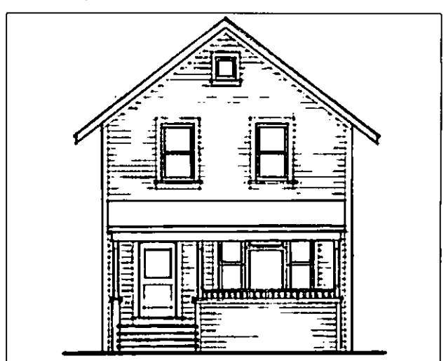
Acceptable Approach, when historical documentation is not available: A folk or vernacular style house with a simplified interpretation of a traditional porch design.
