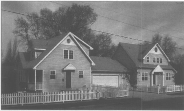
Subdivide larger masses into smaller “modules.” This single-family residence is broken into modules so it will not dominate the scale of the neighborhood. (Lafayette, CO)
