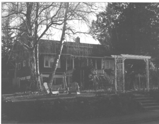
The Anise house c. 1907 is a side gable Craftsman with an ashlar foundation and an exaggerated overhanging roof with exposed rafters.
