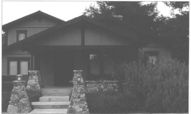
Design a new building to be visually compatible with nearby historic houses. Features such as one-story porch elements which define entries, columns, posts and brackets contribute to the sense of character of the street and add visual interest to pedestrians. (Pacific Grove, CA)
