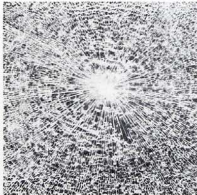
WHEN BROKEN, Vitrolux disintegrates into particles resembling bath salts. Greater impact is required to damage Vitrolux than regular plate glass.
