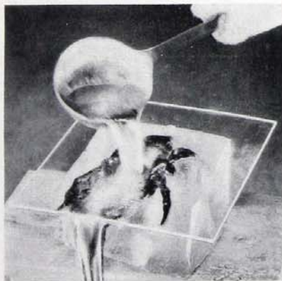
RESISTANCE TO THERMAL SHOCK is illustrated in this test. A sheet of Vitrolux resting on a cake of ice is undamaged by the heat of molten lead.
