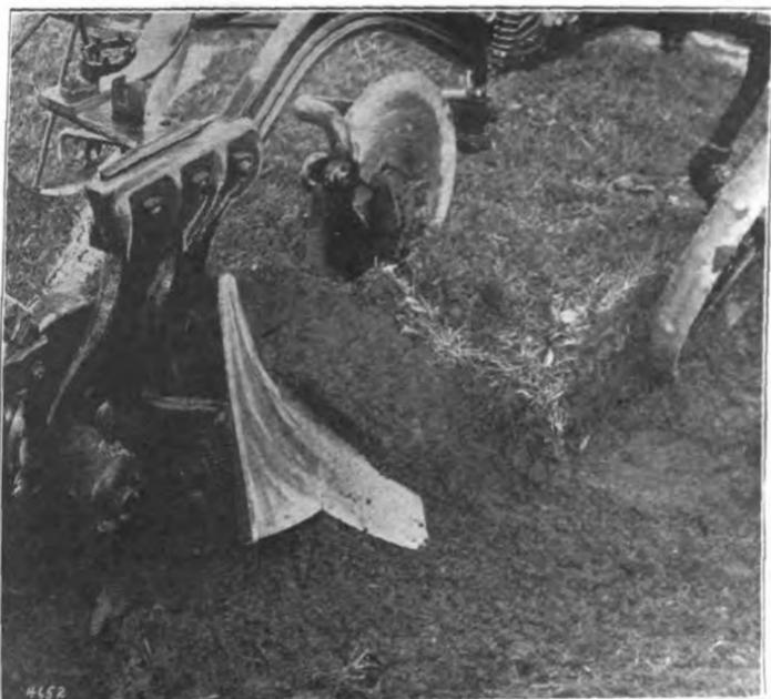
Fig. 7. Shows furrow slice cut further forward than Fig 6
