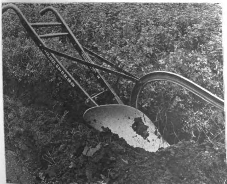
Fig. 8. Plow pulled back in the furrow showing earth sticking to moldboard in spots
