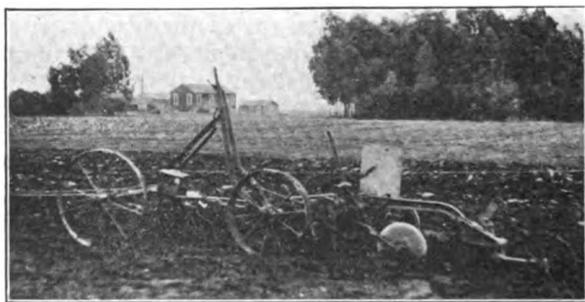
Fig. 1. Showing dynamometer and carriage for controlling width of furrow.
