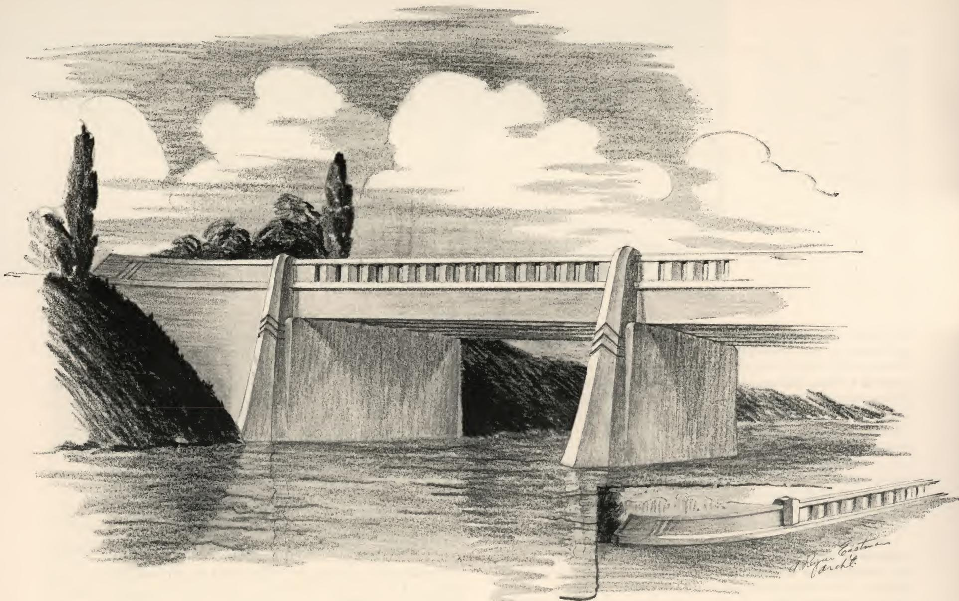
*The design by A. Reyner Eastman is particularly suited to a simply supported deck girder bridge with two openings. The prominence of three supports—only two of which are shown—diverts attention from the duality of two spans. The pier has a definite flare at the bottom for definition and the chevron design serves to describe "support" for the deck girders.*
