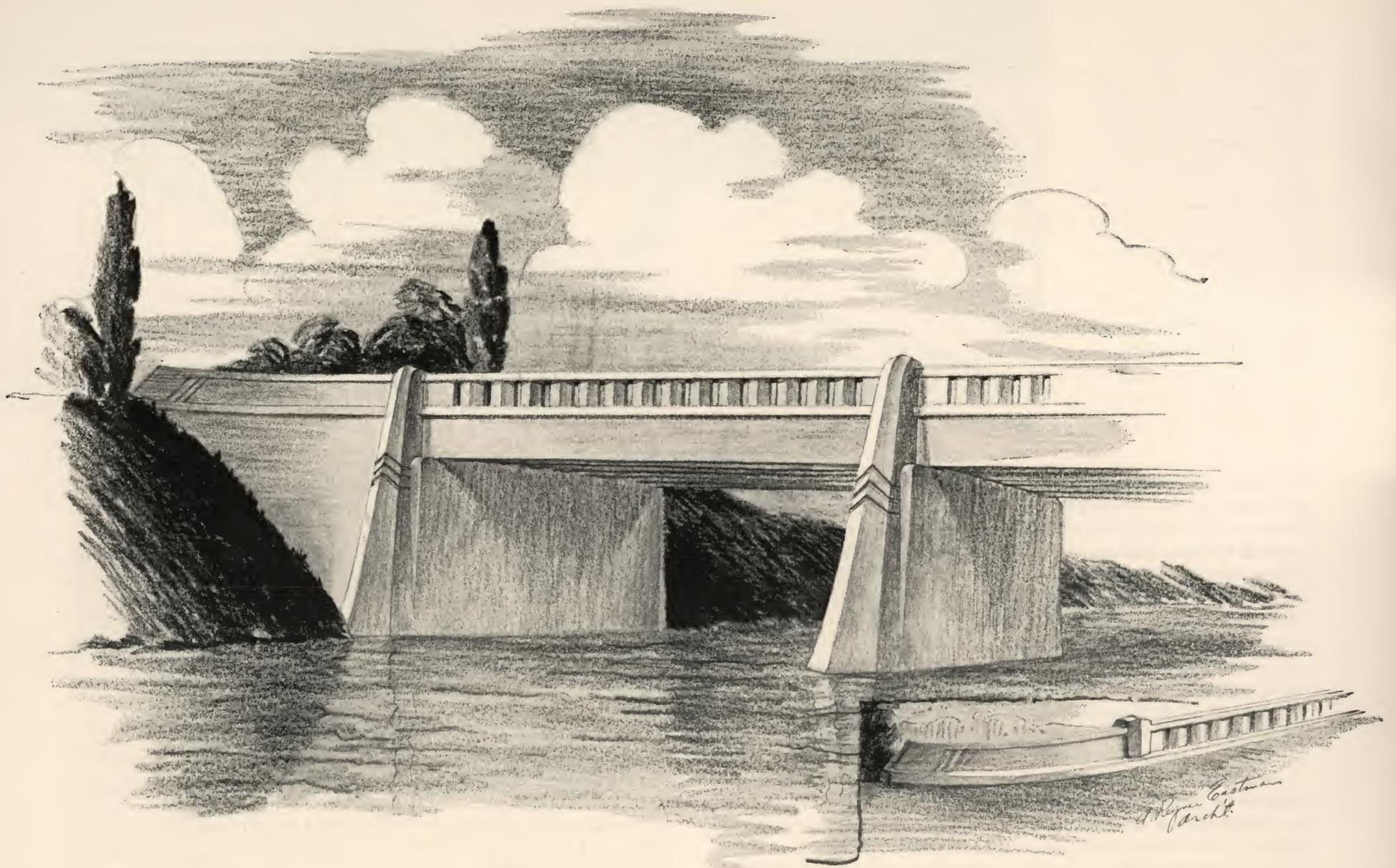
*The design by A. Reyner Eastman is particularly suited to a simply supported deck girder bridge with two openings. The prominence of three supports—only two of which are shown—diverts attention from the duality of two spans. The pier has a definite flare at the bottom for definition and the chevron design serves to describe "support" for the deck girders.*
