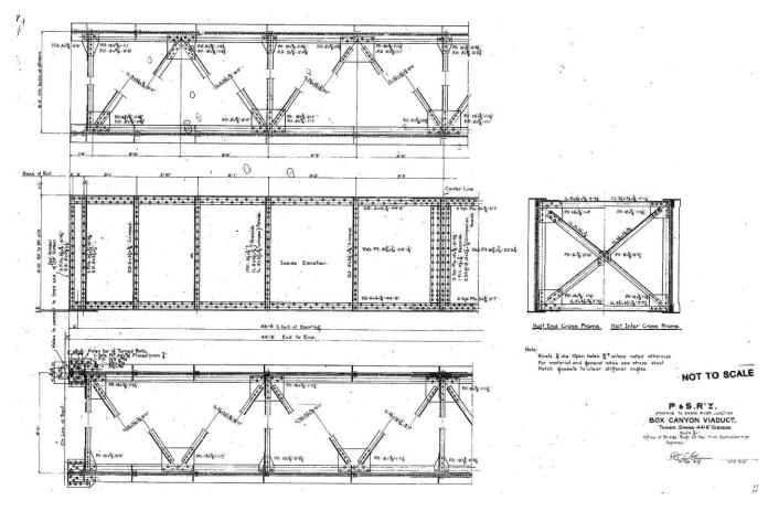
Description: Box Canyon Viaduct, tower span deck plate girders.
