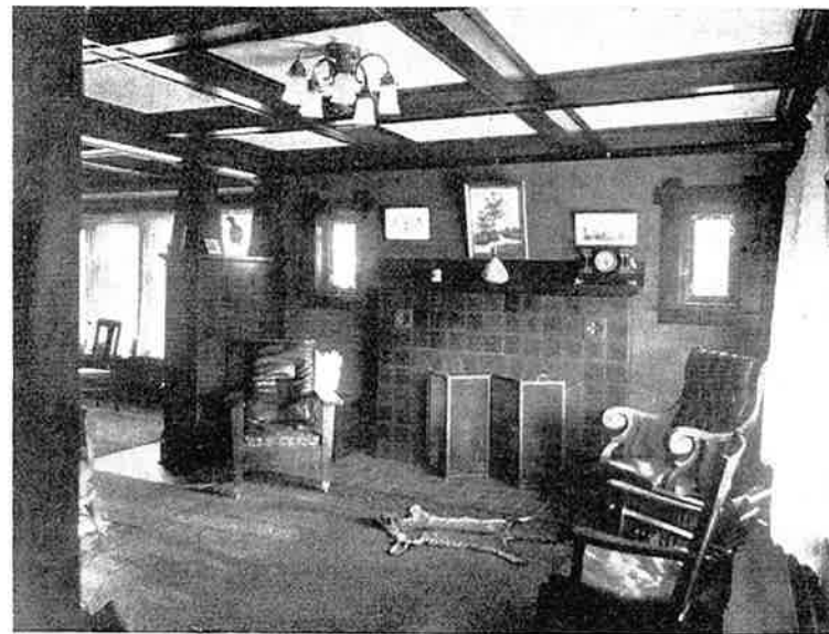
Interior Design 412—A simple but attractive interior, showing the use of square tile for the mantel. The interior woodwork is square design, and the whole is finished in a dark brown with light cream ceilings. The stained art glass used in the high windows on either side of the fireplace lends the touch of color needed to make the whole a most pleasing effect. The walls of this living room are tinted a deep tan, while the ceiling is a light cream tone. The dining room, a glimpse of which is had through the arch, is paneled five feet six inches high with slash grain fir panels capped with a plate rail.
