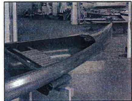
WA-209-1 Bow viewed from starboard amidship. Note mast partner at bow deck
