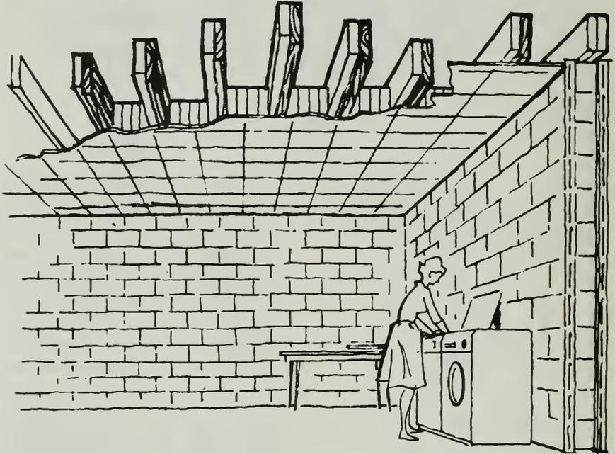
If you need a minimum shelter which will not interfere with an existing corner of your basement, try this plan. It is so arranged that the shelter area can be enlarged at either end, depending upon the size of the basement.
