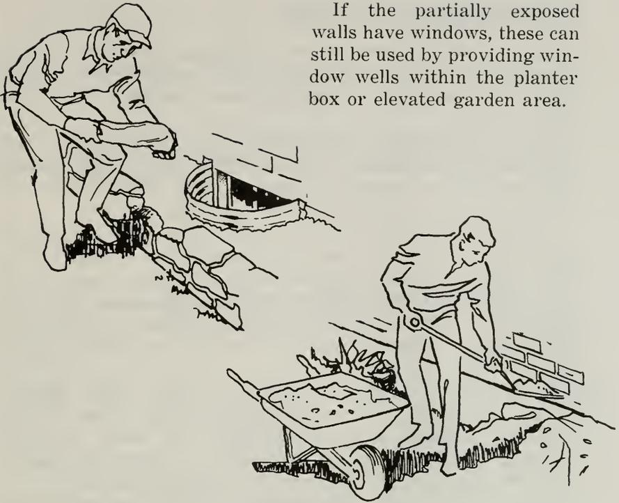
Your basement's PF will also be increased by providing additional shielding to the exposed section. This can be done by piling patio block, sand, earth, cordwood or similar materials against the exposed wall.
