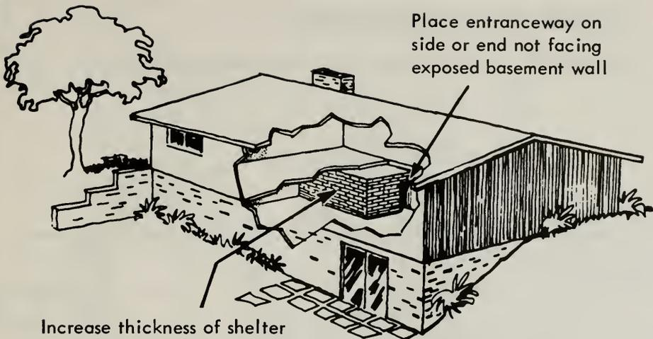
Increase thickness of shelter wall facing exposed basement wall by four inches
