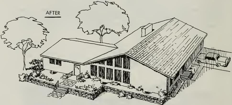
Where basements are not completely belowgrade, here are some additional ideas which can be used to increase the shielding of exposed basement walls. A brick, masonry, or stone planter box along one or more sides of the house will improve protection substantially, and will provide an attractive setting for shrubs and flowers as well. If the partially exposed wall is at the rear or side of the house, an elevated garden could be built with masonry retaining walls.
