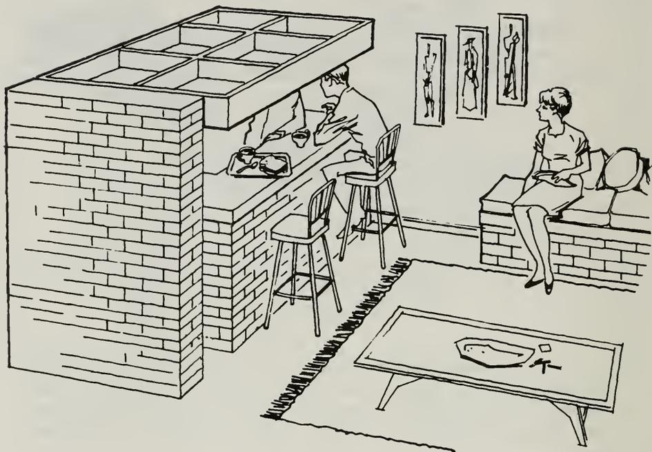
A snack bar built of brick or block can be converted into a fallout shelter in a short period of time by lowering a strong hinged false ceiling to rest on the snack bar.
