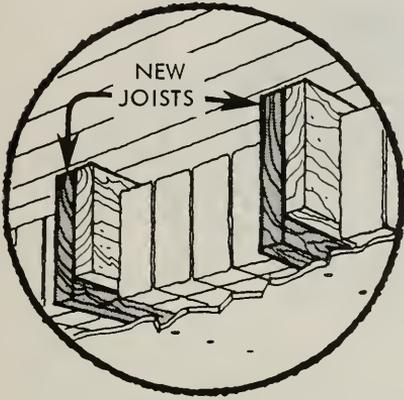
Brick or concrete blocks are packed into the spaces between the 10" and 12" joists; they are supported by the plywood panels.
