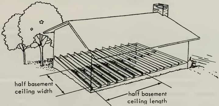
This basement floor plan shows how the additional joists and the filler material might be used in the corner of the basement which furnishes the best fallout protection. To get the most protection out of this improvement, one-quarter of the basement ceiling should be filled with bricks or solid concrete blocks.
