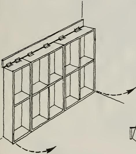
A tilt-up storage unit in a corner of your basement is another approach similar to the snack bar. The top of the storage unit can be hinged to the wall and the unit can be used as a bookcase, pantry shelves, or for miscellaneous storage.
