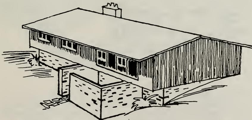
Enclosing your patio area with a solid masonry screen wall will give you privacy for lounging and cook-outs, and will provide a barrier shield to increase the PF in the basement area.
