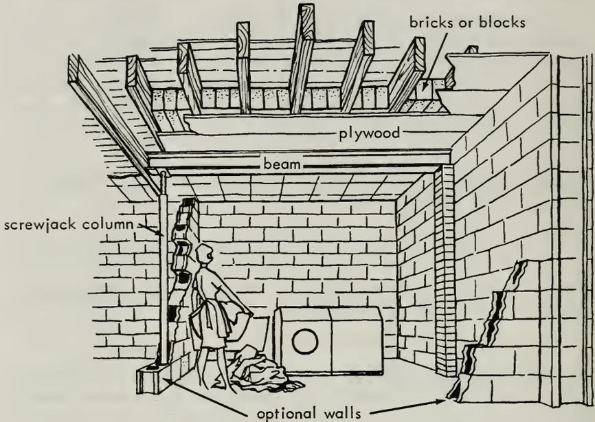
Here is a shelter which can be permanently installed in the basement of your home without affecting the use of the basement in any way.
