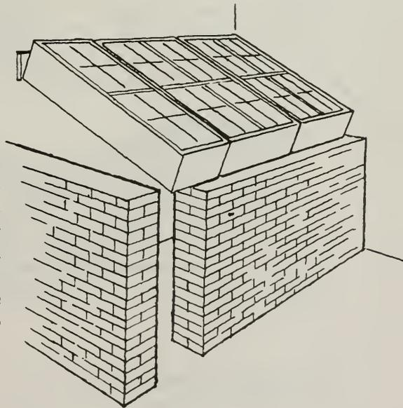
In an emergency, the storage unit can be tilted so that it rests on a wall of brick or concrete blocks stored for just such as emergency. Additional bricks or blocks can then be placed in the storage unit to provide an overhead shield.
