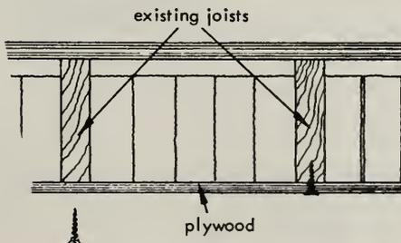
In fastening the plywood sheets to the joists, nailing is not enough. Nails will pull loose. Use two-inch screws in the manner shown here.
