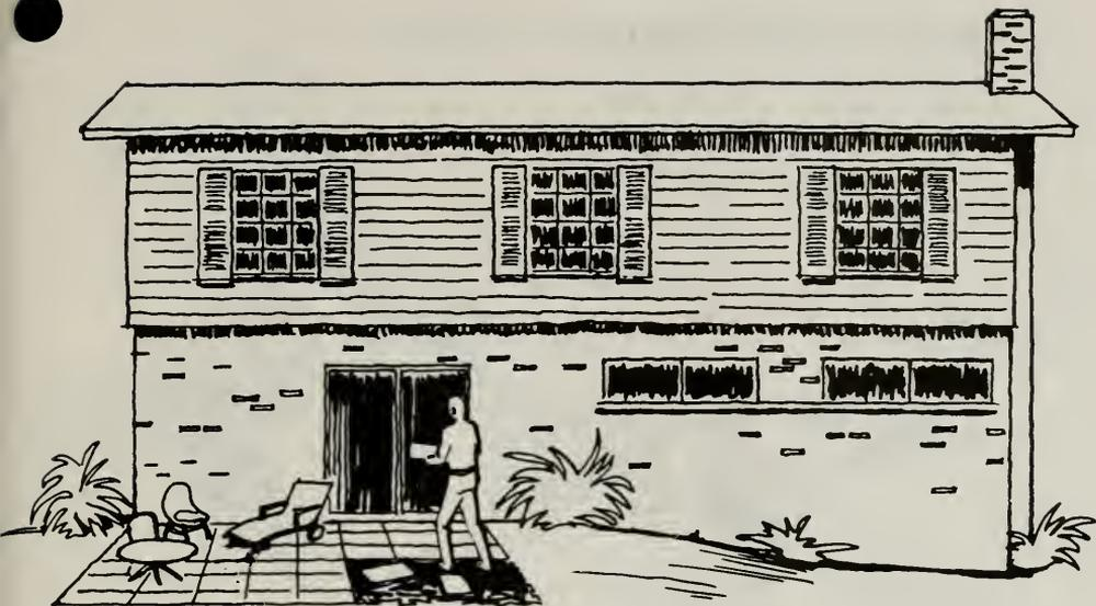
A patio of brick or concrete block supported on a bed of sand will provide a ready source of shielding material which could be quickly removed for use in an emergency. See Plans D, E and F.
