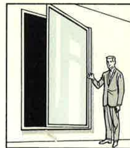
Pivomatic as a side inswing window. Easy to clean.
