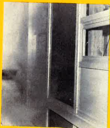
WINDOW UNIT. 11'-3" x 18'-0". The window unit tested was complete in every detail to that proposed for the Alaska Mental Hospital.
