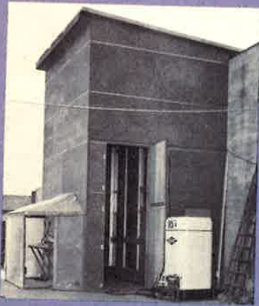
TEST CHAMBER CONSTRUCTED by Fentron. It is equivalent to (2) floors of the building, accommodating an actual job size unit for testing.
