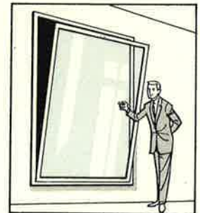
Pivomatic as a bottom inswing window. Controlled ventilation.
