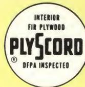
This trademark—stamped on the panel back—identifies the unsanded construction grade of Interior-type plywood bonded with water-resistant, but NOT waterproof, glue. Use Plyscord for hidden structural uses—wall and roof sheathing, panel backing, subflooring. Plyscord is also used as a one-use concrete form panel, then re-used as subflooring or sheathing.
