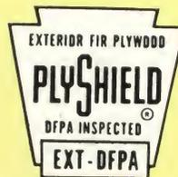
This trademark—stamped on the panel back—identifies Plyshield, the versatile "one-side" grade of Exterior-type Douglas fir plywood with 100% waterproof bond. The panel face is of the highest appearance quality; the back contains certain limited wood characteristics such as knotholes. Use Plyshield for exterior siding, outdoor storage units and for inside uses such as drainboards, showers, etc., where water or moisture is encountered.
