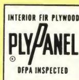
Stamped on the panel back, this grade-trademark identifies Plypanel the "one-side" grade of Interior-type plywood. The face is smooth, paintable; also with selection for uniformity and appearance, beautiful light-stain finishes may be used. The face of the panel may contain neatly-made repairs. Use it indoors only—for wall paneling, built-ins, and other uses where only one side of the panel will be in view, as well as for the finest linoleum base.
