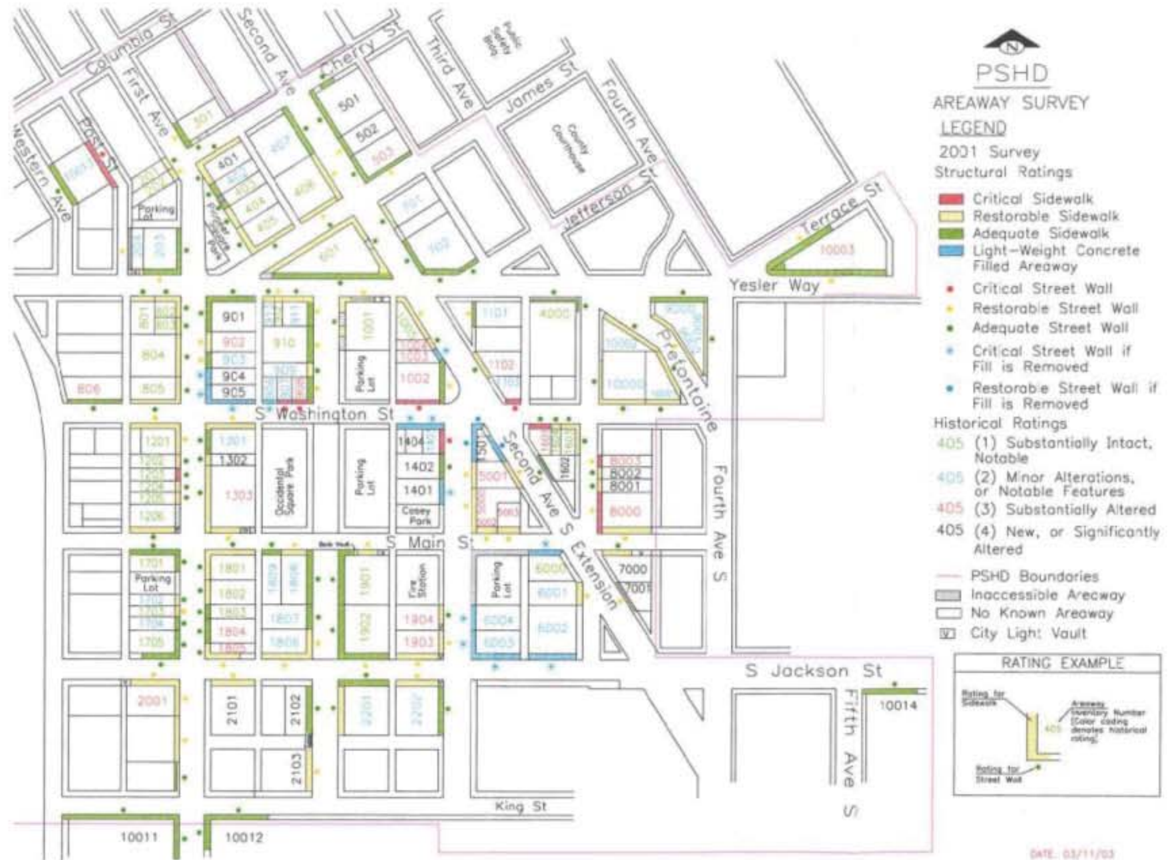
Map of Pioneer Square's Areaways and their Structural Ratings from the 2003 SDOT Pioneer Square Historic District Areaways Hazard Mitigation Study
