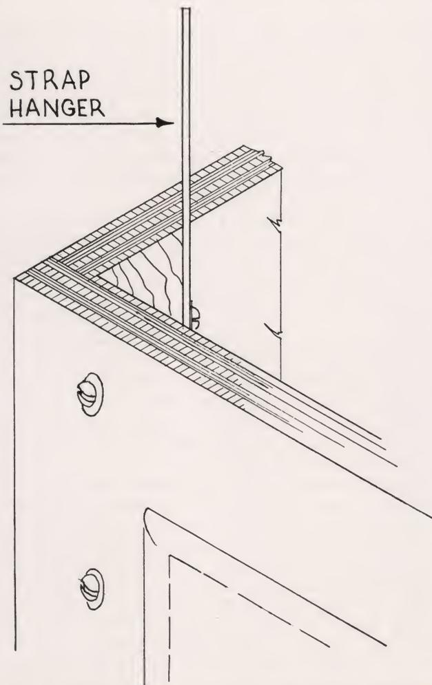
*Hanging Cabinets from Ceiling Beams Eliminates Cracks at Ceiling*
