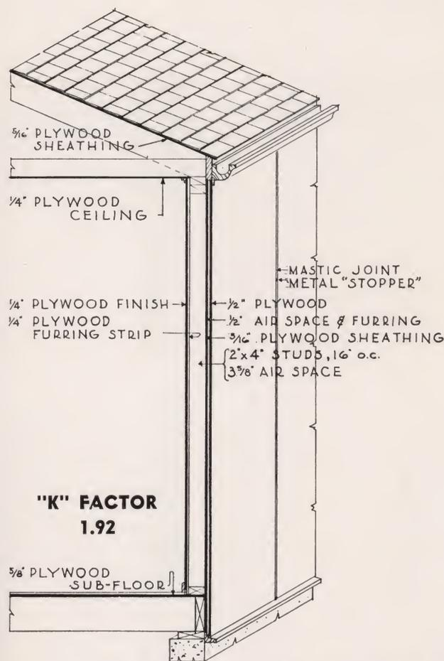
The third wall section shows a system which produces a simple unbroken wall surface which has been the aim of designers since the ancient Greeks patiently ground their stones to eliminate the appearance of a joint.
