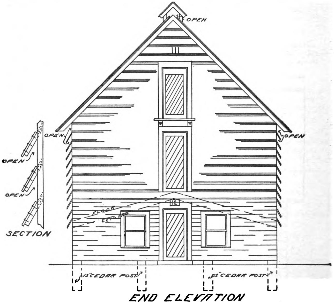
essary to put a slatted partition on both sides of the floor ridge if the house is filled full of corn. There are two windows in each end and the hog doors are hung with pins so they swing either way and the hogs open them going or coming. A pin at the
