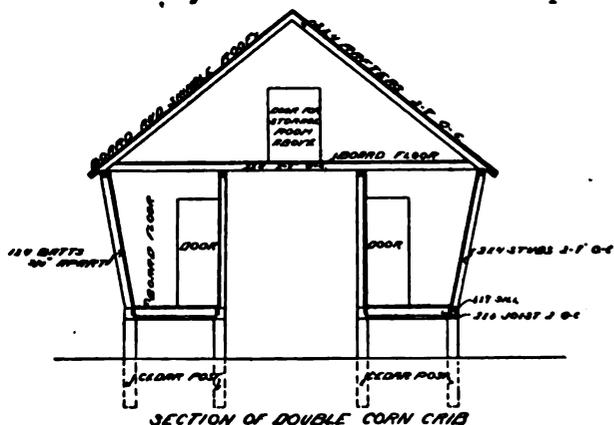
between the two cribs makes a convenient place to store a couple of wagons. The doors being at the end, the center space is left free for this purpose. A good many cribs built on this plan have the doors inside opening from the center passage, but if the space is desirable for wagon storage
