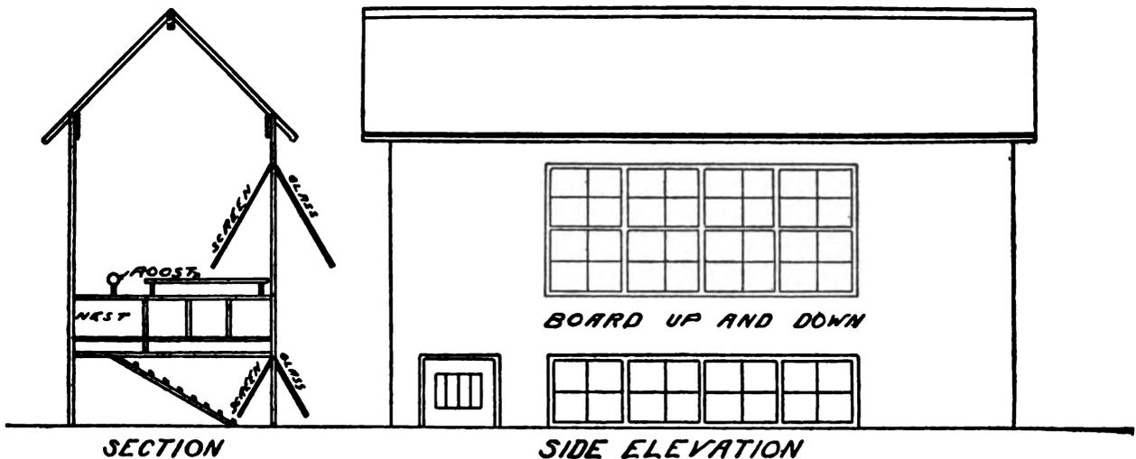
house. This little house is four feet wide and twelve feet long with a scratching shed the full size on the ground under the floor. This space underneath is two feet high and the windows should extend well across the front side.
