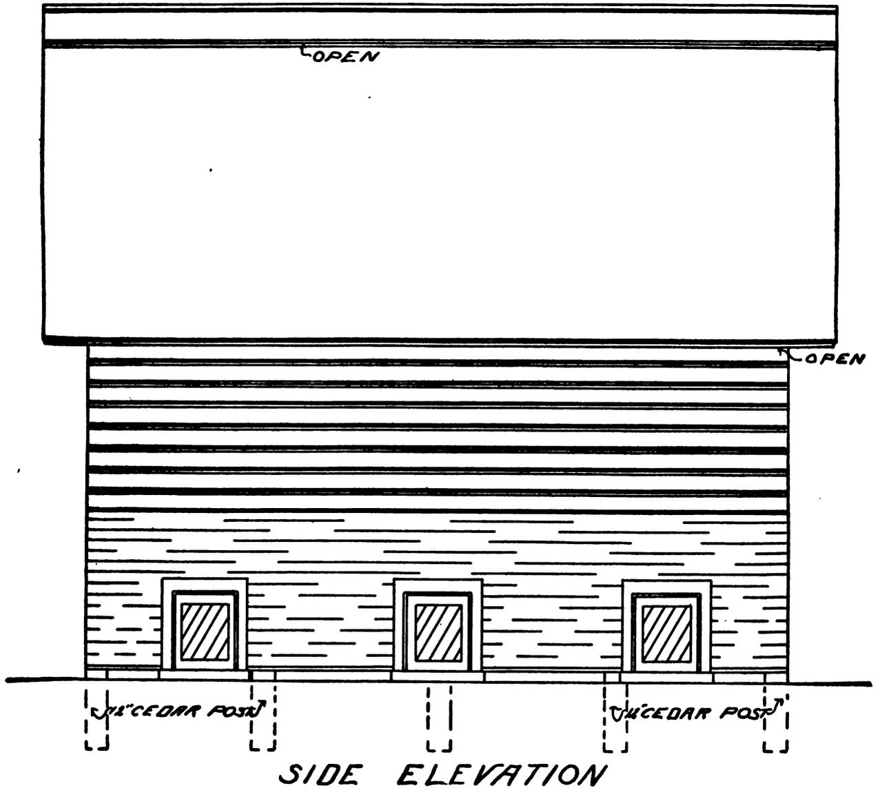
The building is set up from the ground about a foot on posts and pens are made seven feet head room in the middle over the alley and the floor slopes to about five
