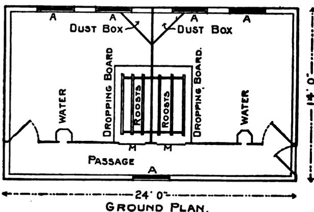
in front of the roosts from this passageway to facilitate cleaning. It is not necessary to enter the scratching room very often because most of the attention may be given from the alleyway. With the exception of the space occupied by the dust boxes the whole floor, except this passageway, is given over to scratching purposes as the roosts and dropping boards are elevated so the chickens can work under
