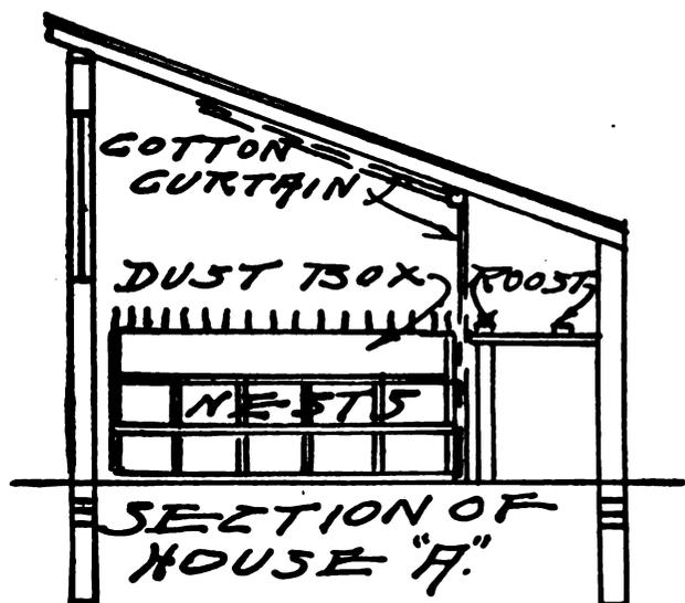
Some poultrymen cover all the openings with cotton and have glass sashes inside that they may slide shut at night or during extremely bad weather. When the cotton ventilators are made right and kept right the air in the poultry house will be good.
