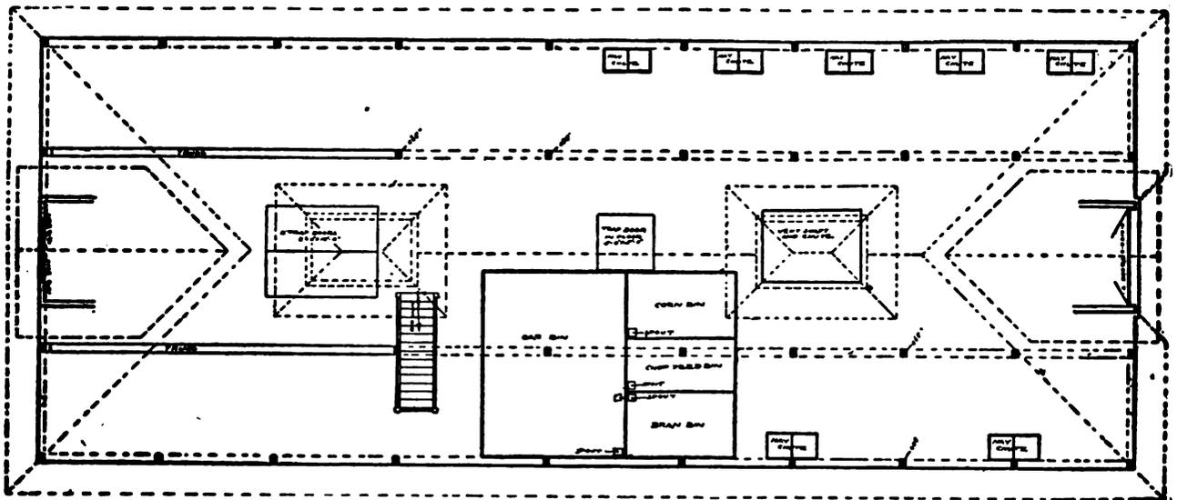
trap door for throwing down hay and bedding, and also for the hoisting of hay from the hay wagon in stormy weather.
