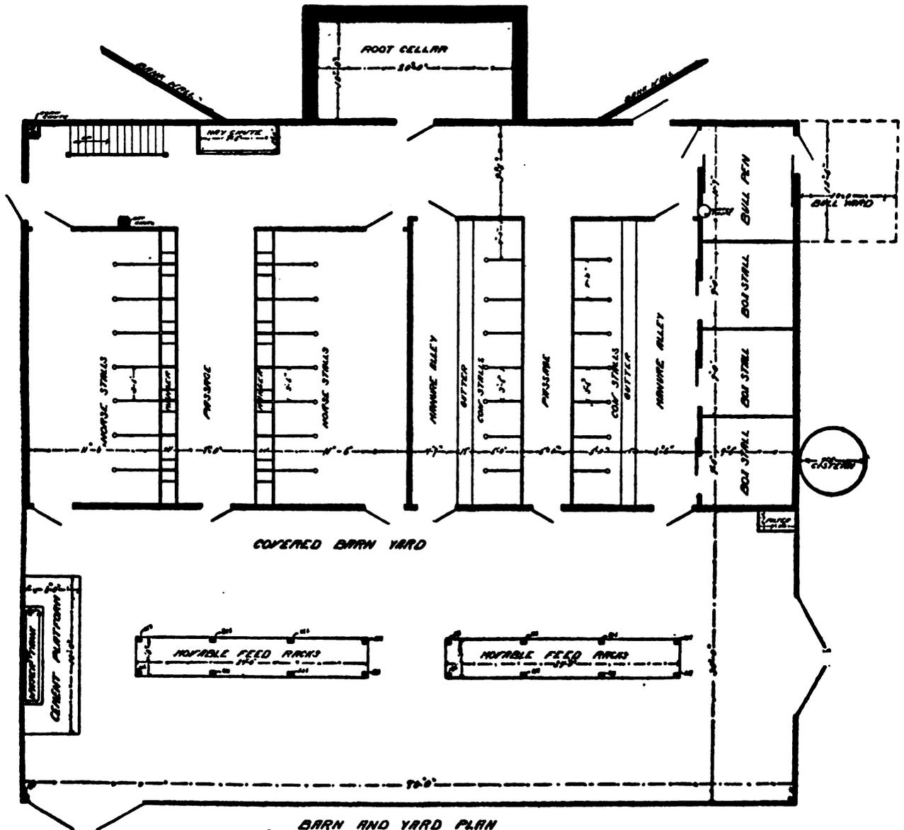
With a cistern and a windmill the water tank is kept supplied all the time so the cows may run to it when they want to. The stable floor should be about two feet higher than the floor in the covered barnyard. This gives an eight foot ceiling for the stable and a ten foot ceiling in the yard.
