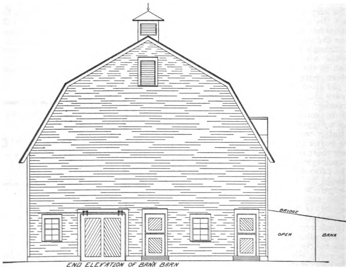
peculiarity of this style of barn is what is commonly termed a double threshing floor. In some of the larger ones the getting the grain to the machine. The bridge from the bank to the ground floor must be stronger than common barn
