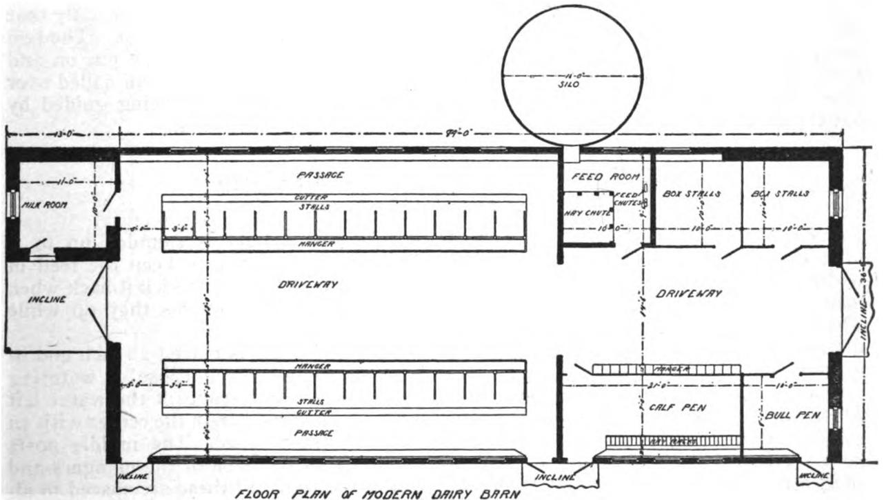
out altering the width or the general plan. Placing the silo near the middle of the building saves carrying the silage more than fifty feet which is a great saving of
