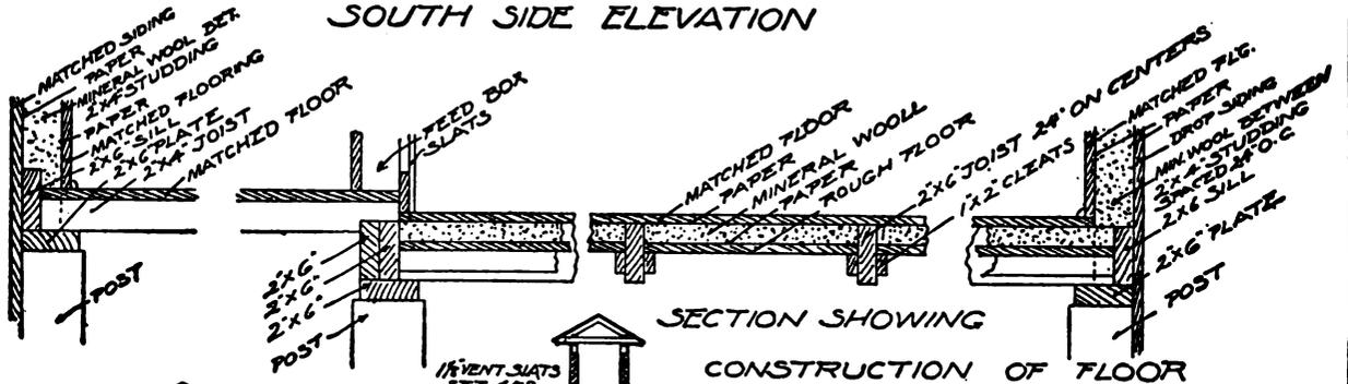
SECTION SHOWING CONSTRUCTION OF FLOOR
