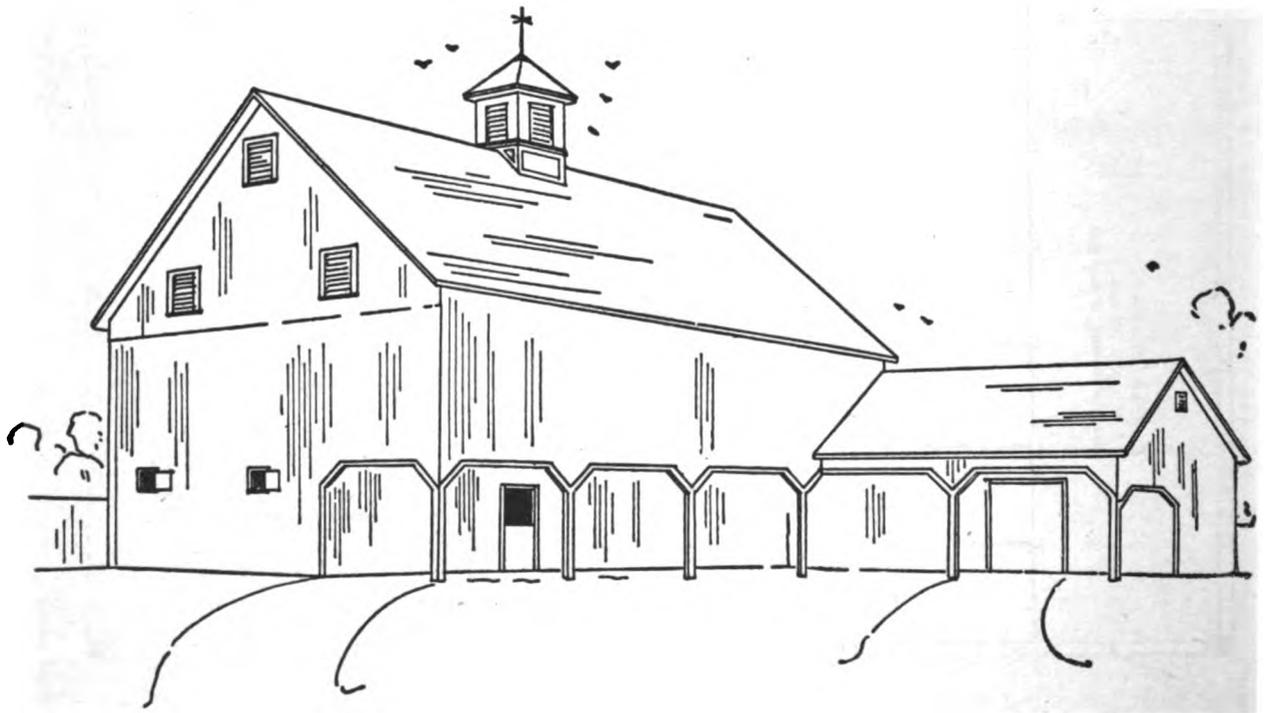
five feet to the comb. On the north is a low sheep shed forty feet long by fourteen feet wide, and extending east of this is another low addition twenty-six feet long by eighteen feet wide, the north half of which is used for horse stalls, hog house and corn
