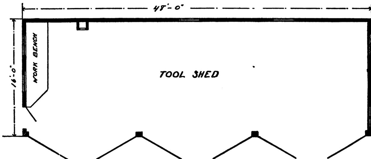
but you don't need so much height to the back end. The doors in this plan are ten feet high and the cross girts are the same height because it is sometimes necessary to move the machines lengthwise of the shed and the same head room is then needed. A truss is formed at each bent with the rafters to prevent the building from spreading. The two by four nailers shown
