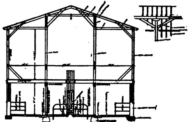
The stall floors have a gradual slope to a shallow gutter at the rear of the stalls and this gutter has a gradual slope to a drain tile to carry out all liquids to a cistern under the compost pits at the end of the barn. Calf stalls and loose stalls for dry stock and bull are arranged about the
