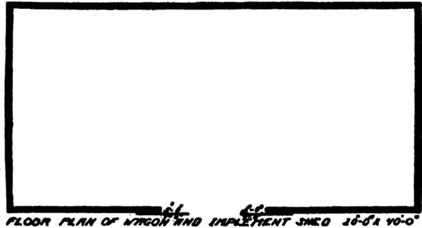
gives an opening ten feet wide, which is very good for small implements, but some binders require about sixteen. The door entering an implement shed must be high enough to let in the highest implements used on the farm, and there must be no cross timbers inside lower than the top of the door. A binder with a reel on takes considerable room.
