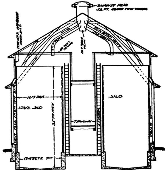
SECTION SHOWING SILOS AND VENTILATION FLUES
