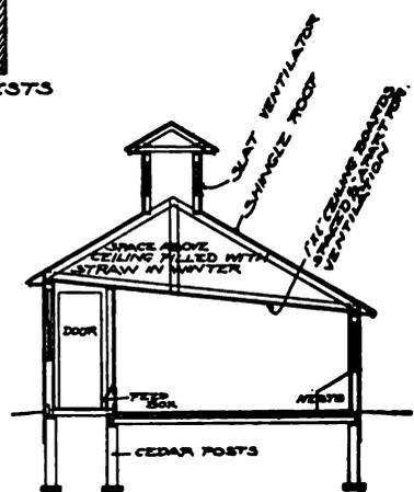
The building is sixteen by thirty feet and contains one general room with a passage, which is also a storeroom for feed, along one side and across one end. All the principal construction details are fully shown in the detail drawings.
