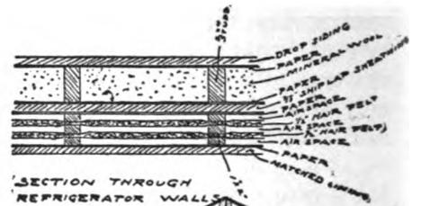
SECTION THROUGH REFRIGERATOR WALLS
