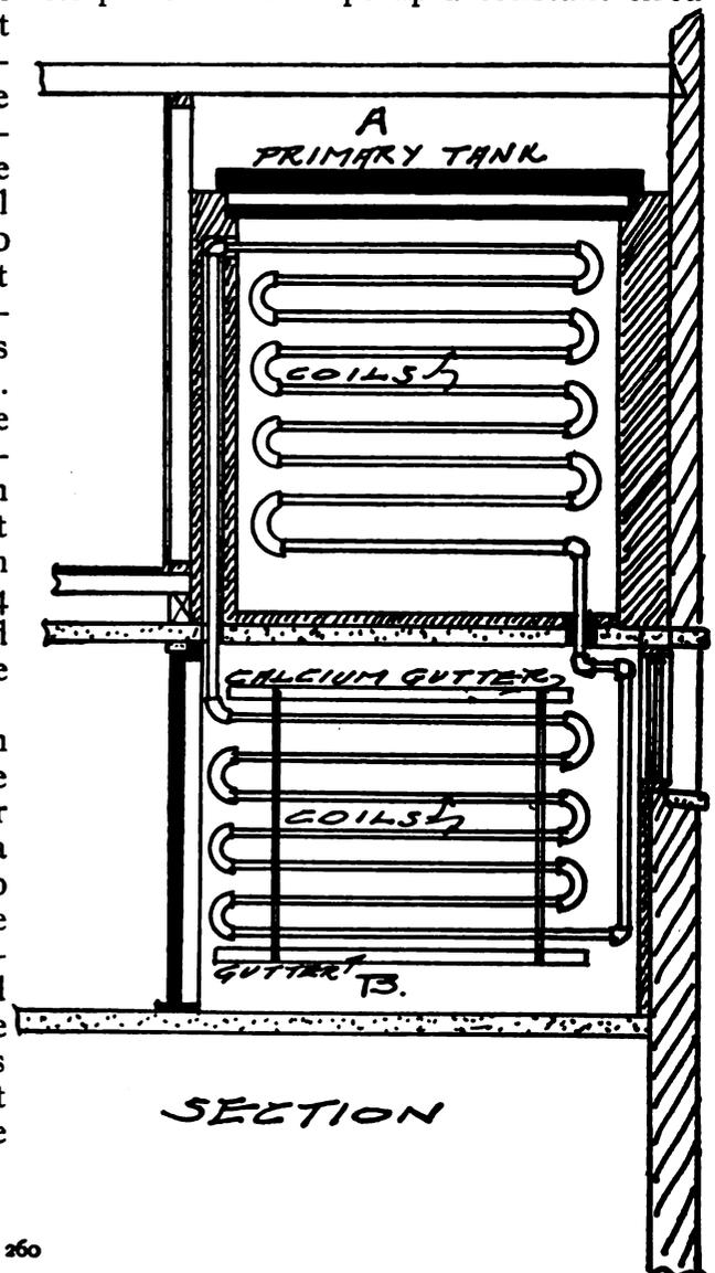
lation whereby the pipe in the lower room is kept cold and the degree of cold is regulated by the size of the cold storage room, the area of pipe surface and the amount of
