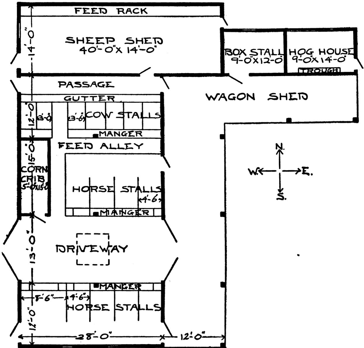
crib, the corn crib being built over the hog compartment. The south half of this extension is an open shed. Also an open shed extends along the east side of the main building and is equipped with mangers for six horses to be used when extra teams
