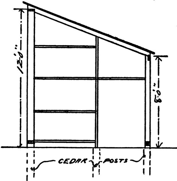
long and ten feet six inches wide. It is built of two by fours for framing, covered with boards twelve feet and sixteen feet
