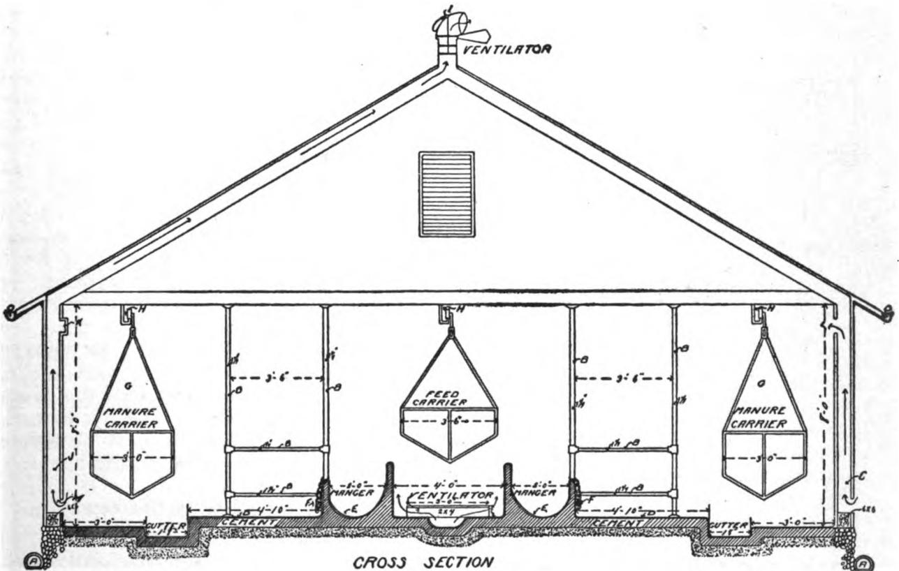
ing paper around all such places to prevent air openings. It is not intended to use the loft over this stable for storage or any purpose but it is better to build the loft so that it may be swept occasionally to clear out the dust. A window is placed in each gable for the purpose of causing sufficient
