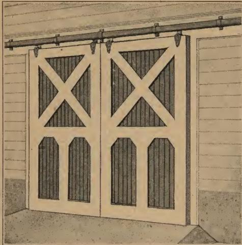
Double Sliding Driveway Doors for the ground floor of "HONOR BILT" barns are 8 feet 2 inches by 8 feet in size and 1½ inches thick. For entrance with team and load into the mow, these doors can be furnished 12 feet 4 inches by 12 feet in size, with a small door built in for personal access.
