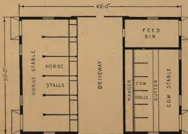
This floor plan is suitable for barns with a large driveway in the center running through the side of the barn.
