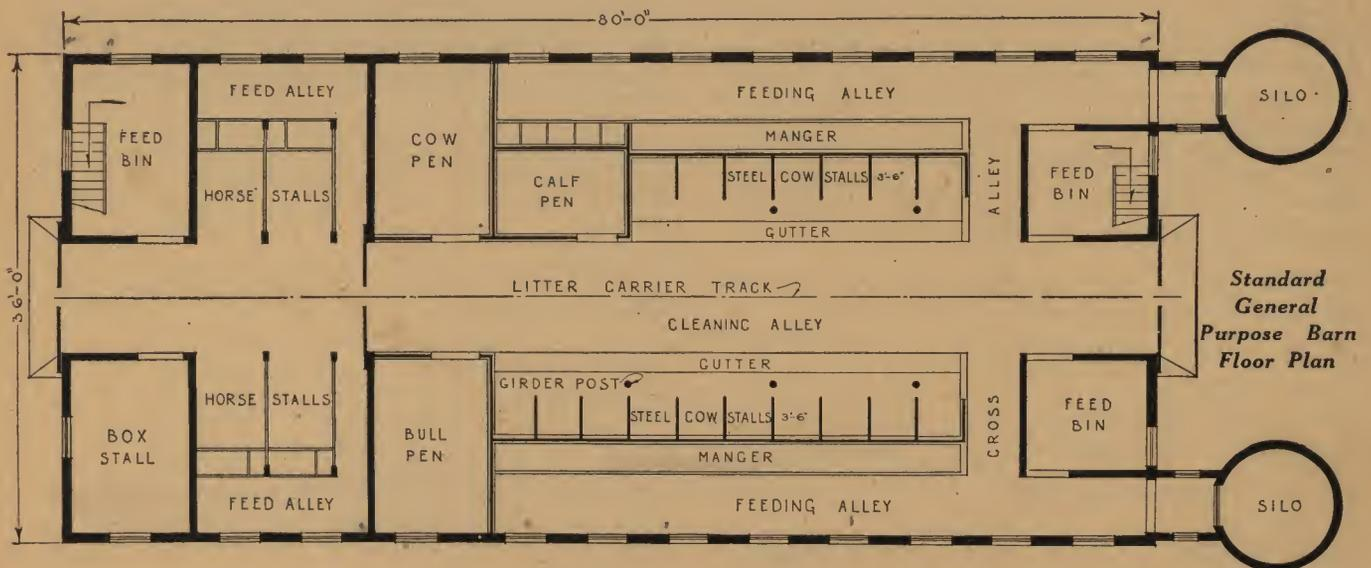
Combination horse and dairy barn floor plan arrangement. This floor plan is suitable for all barns with an 8-foot driveway running lengthwise through the barn.
