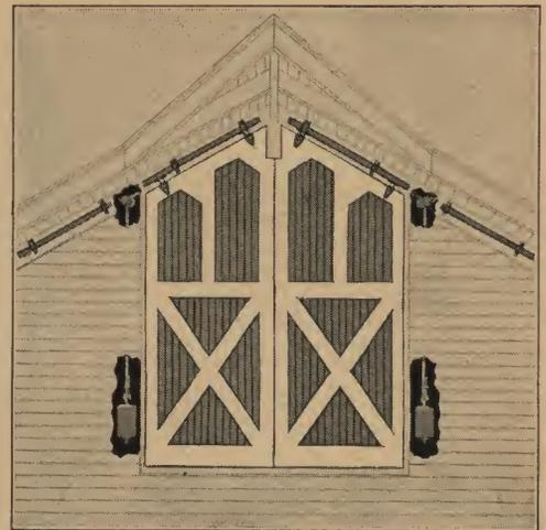
Two kinds of gable hay doors—the gable sliding type illustrated and the hinged drop leaf door—are used on "HONOR BILT" barns. The counterweights for the sliding doors are best made of concrete and are to be furnished by the owner. The hinged door can be easily opened and closed with the aid of the hay carrier. The doors are 9 ft. 4 in. wide by 12 ft. 8 in. high and 1½ in. thick.
