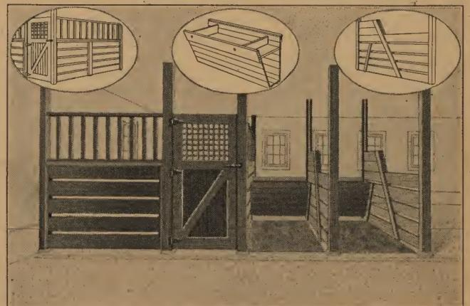
Box Stall, Single or Double Horse Stalls and Mangers. Stall partitions are made of heavy 2-inch planks spaced 2 inches apart. The factory made door for the box stall is furnished ready to hang in place. Prices on material for stalls quoted on request.
