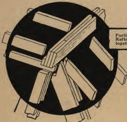
Purlin Plate, Truss Posts and Rafters, showing how they fit together.
