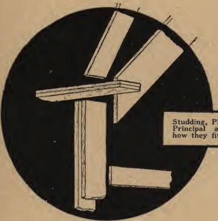
Studding, Plate, Rafter, Truss Principal and Tie, showing how they fit together.
