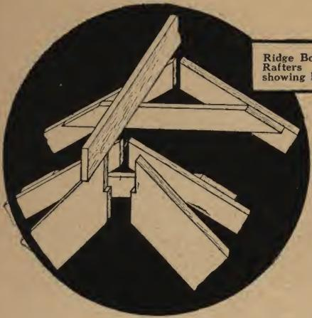
Ridge Board, Truss Principal, Rafters and Collar Beam, showing how they fit together.
