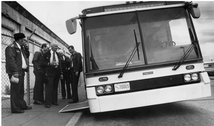
[Figure 33] Seattle, WA. In 1975, Metro bus drivers inspected the Rohn Industries Transbus prototype air suspension system under development for potential production in the 1980s.
