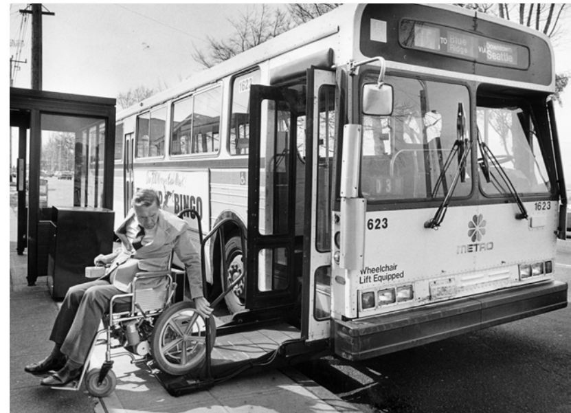
[Figure 34] George Tuner, chairman of the Metro Elderly and Handicapped Advisory Committee, demonstrates a wheelchair lift on a Metro bus.
