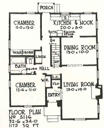
PLAN No. 5116 Size 32'-6" x 34'-0" — Area 1175 sq. ft. Early American styling and careful planning have been combined to produce this comfortable house with a basement and large attic.
