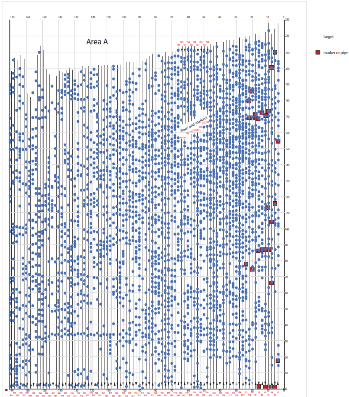
Figure 5. GPR lines and GPR targets for Area A. Higher-amplitude targets are plotted in red. Targets that may be associated with burials are marked in blue.
