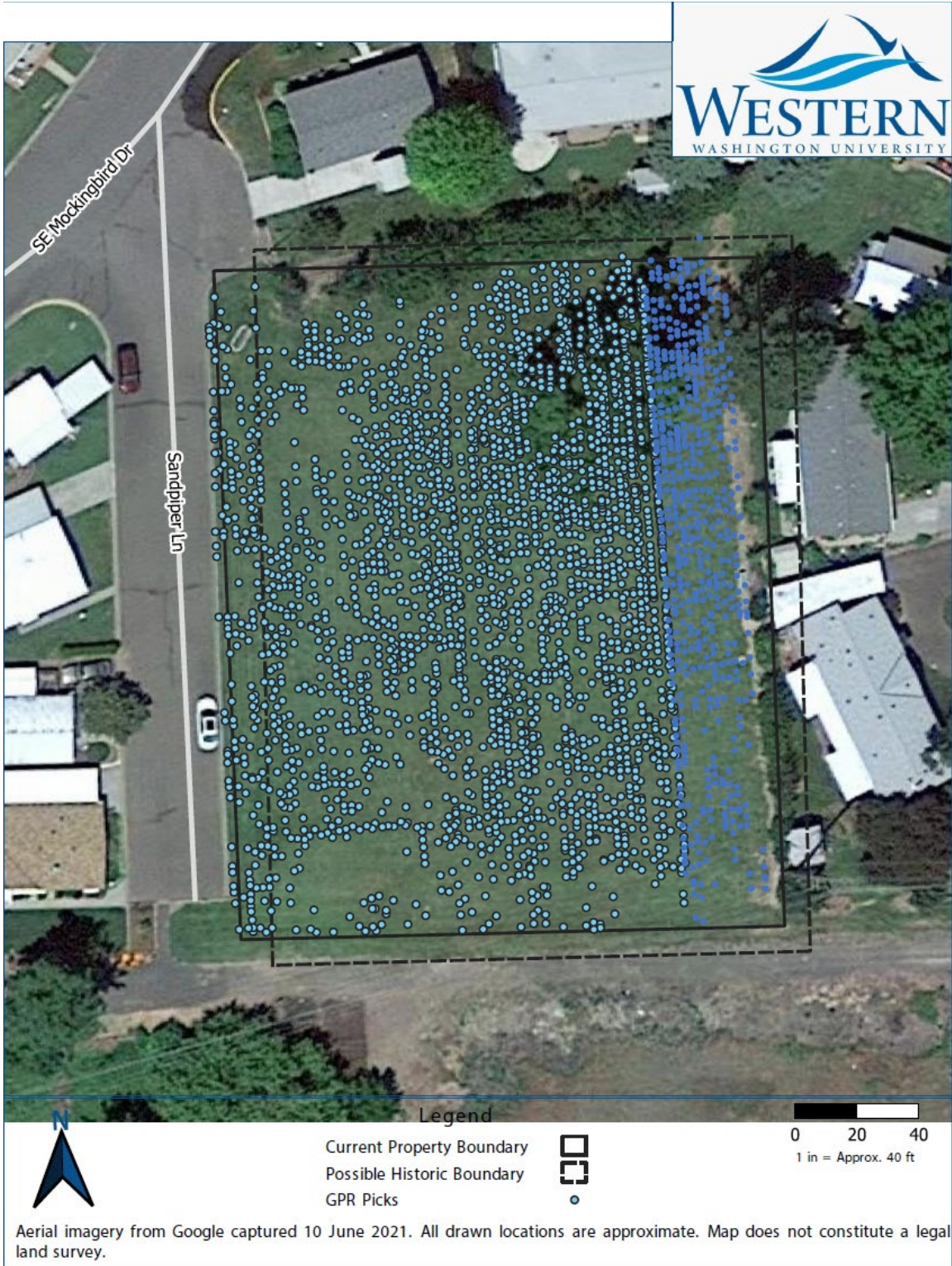
Figure 6. GPR targets plotted on air photo map in GIS database. Darker blue targets on East side were interpolated without GPS data. All other targets located using GPS coordinates from the collected GPR data.
