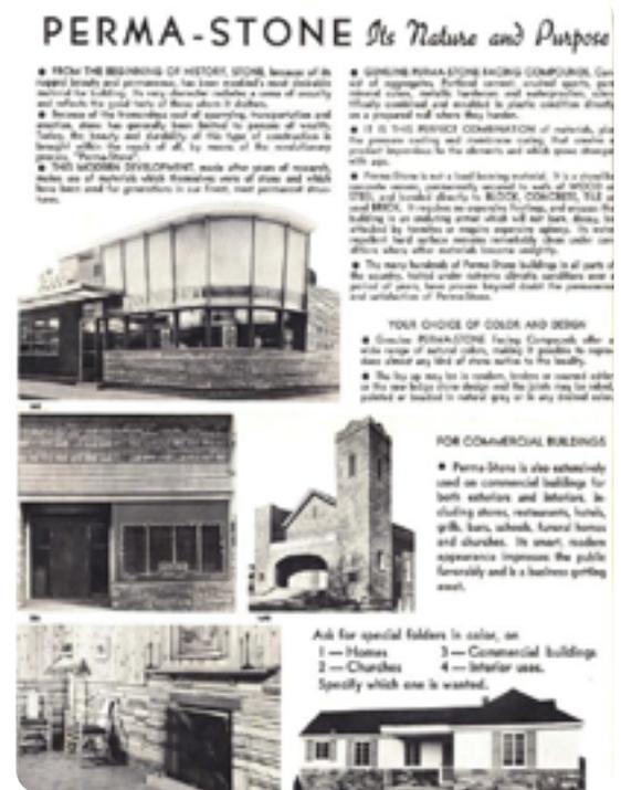
Formstone, developed in 1937, similar to Perma-Stone a cementitious mix applied in layers to lath or directly on masonry. Formstone installers used rollers to create the finish surface. A bond breaker of wax paper or other material kept the cast aluminum rollers from sticking. The transition from stone as a load bearing material to a purely decorative material occurred before 1930, but the visual characteristics and the means of installation evolved.
